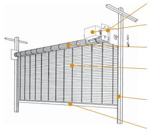
**BRACKETS** - Steel with powder coating in Gray. Bolt to guide assembly and support counter-balance shaft and curtain.
